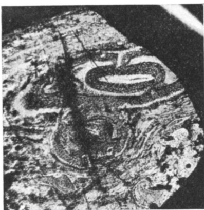
FIG. 2.—Section ( \times 170 ) crosswise to the bedding, from Pennsylvania anthracite. Shows large, wrinkled spore exines found in the duller layers.
